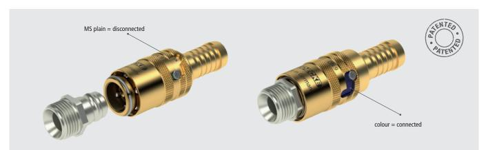
The disconnecting process can be performed blindly due to the forced guidance of the locking sleeve. However, this requires a deliberate manual unlocking effort. An accidental or unintentional disconnection is almost impossible.
